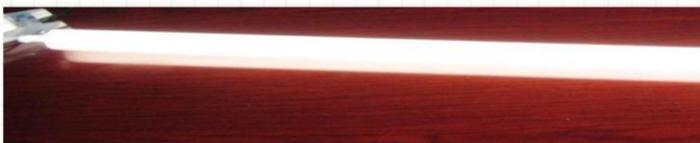
No LED dies are seen after diffuser film is applied.
